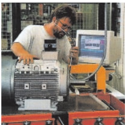
Noise level testing and final electrical inspection of a three-phase motor.
