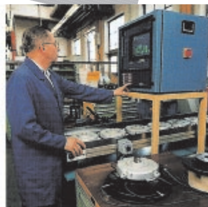
Electronic monitoring of the finished dimensions of a motor end shield.
